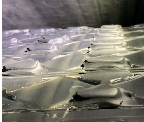
Figure 10 Lagging Failure from Tread Root Location
