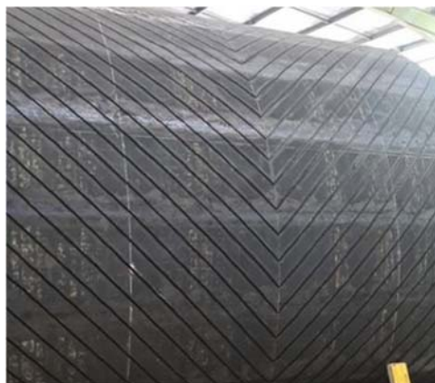
Figure 12 Herringbone Pattern Lagging
