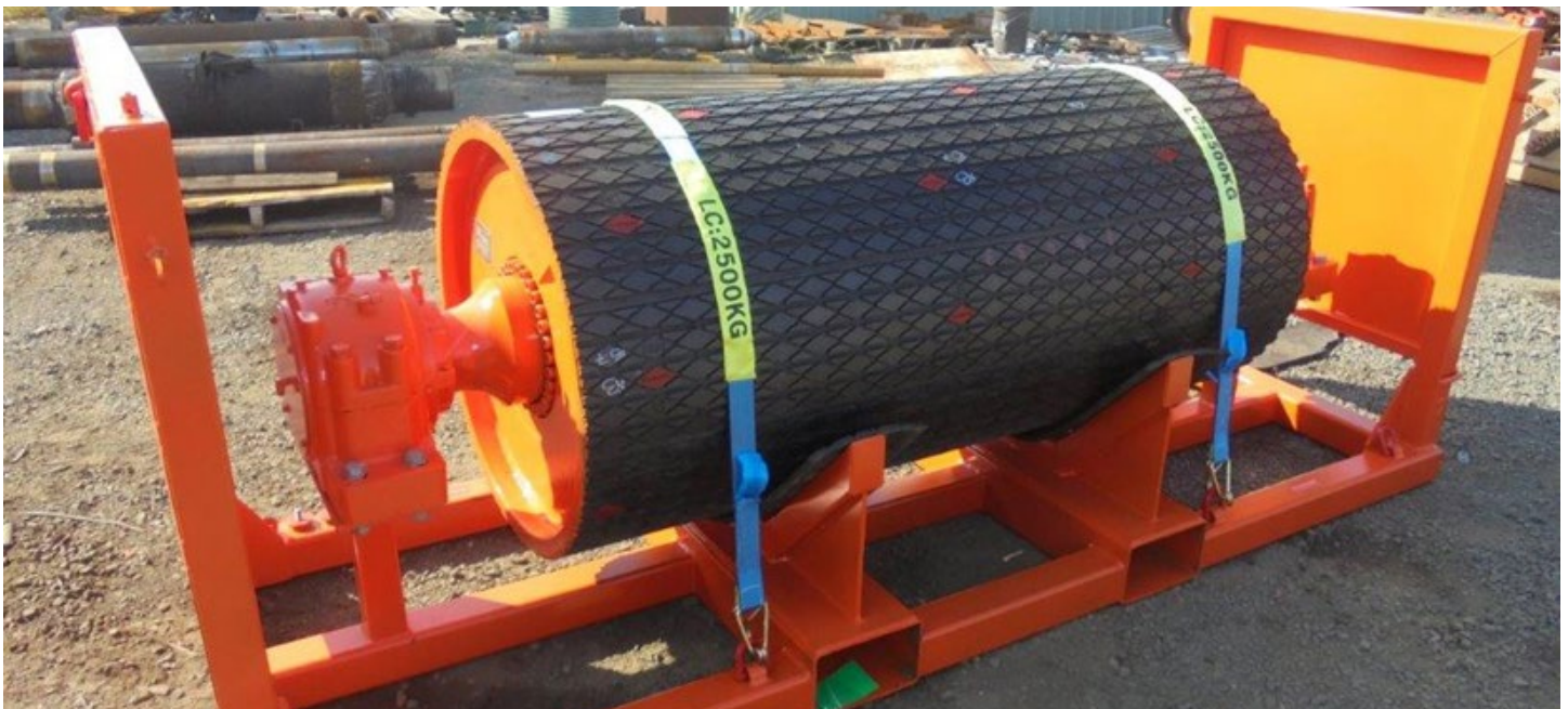
Pulley well secured in the HEME cradle – note the “RED” diamonds in the lagging that indicate “FRAS” lagging
