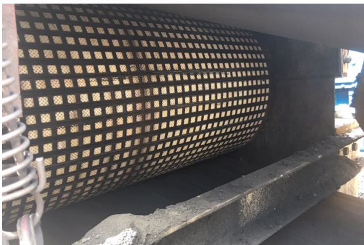
Elastotec HV Ceramic lagging operating at Curragh – note all tiles in place – no tile debonding guaranteed by Elastotec
