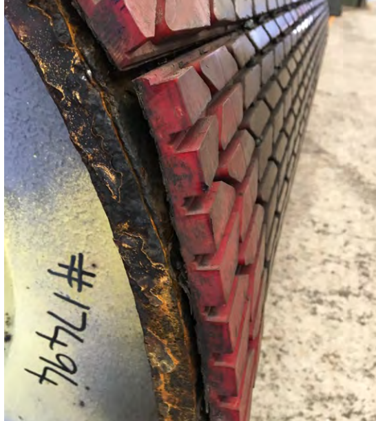
Photo #10. Edge lifting of cold vulcanised PU lagging operating in a coal wash plant.
