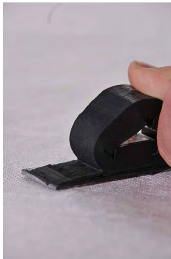
Photos #4, #5 and #6. 100% Rubber Tear bond obtained with hot vulcanised lagging application and tested on EVERY Elastotec lagged pulley.
