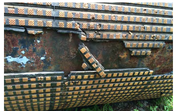
Photo #16 and Photo #17. Corrosion and lagging debonding at joints between cold vulcanised lagging strips due to water penetration.
