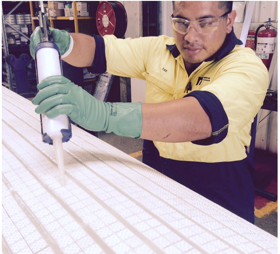
Grouting the DBCL to finish the lagging
