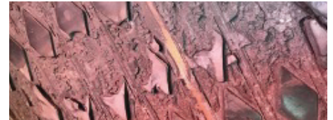
5MW, Coal, NSW, Australia. Rubber melting
