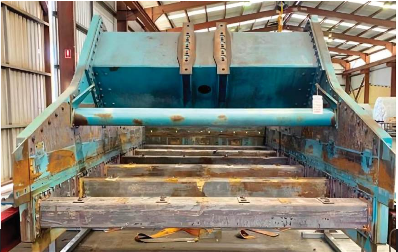
Vibrating screen being refurbished with screen beams ready for rubber lining
