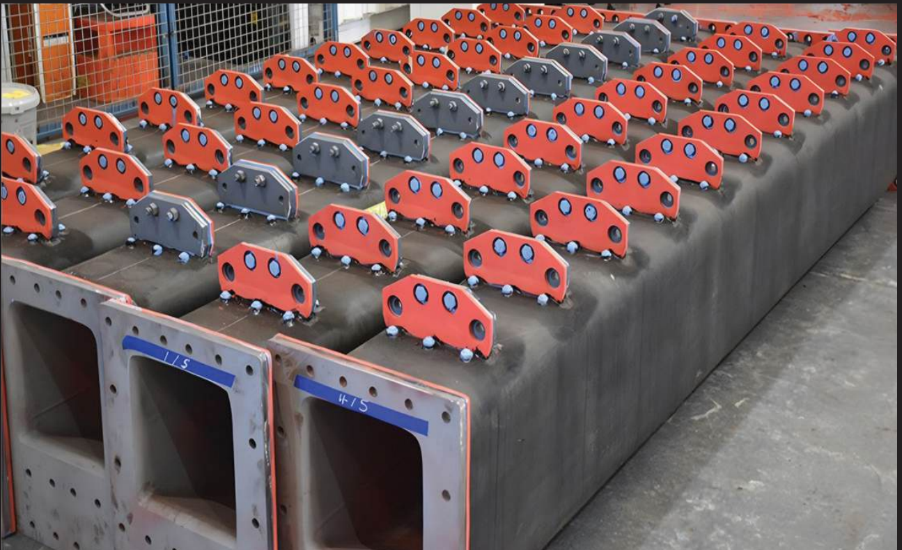
Screen beams that have been cold bond rubber lined
