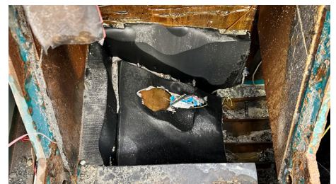
Figure 1. CG12 rubber floor liners show wear and damage after six months in service.
